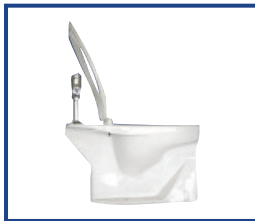
External check hinge stops seat 11 degrees beyond vertical to minimize damage to flush valve
